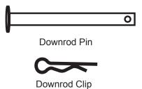
10. Depending on the length of downrod you use, you may need to cut the lead wires back to simplify the wiring. If you decide to cut back the lead wires, it is suggested that you do so in the following manner: Take the lead wires and make sure that you have pulled them all the way through the top of the downrod and measure 8 in. (20 cm) of lead wire, and then cut the excess wire off with wire cutters (not included) (Fig. 10).
